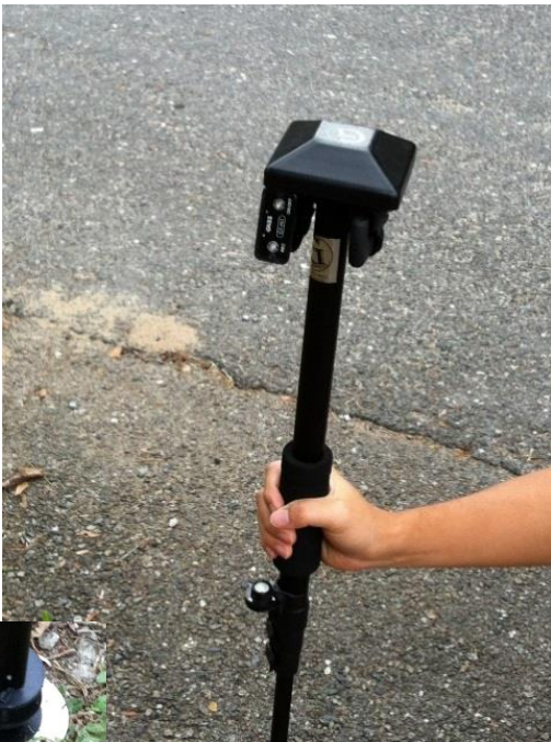
Figure 1: G1-m1™ Mobile System on a Pole over a GCP
