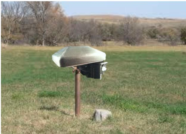
*Figure 6: G1-m1™ System over a monument pillar in a static data acquisition session*
