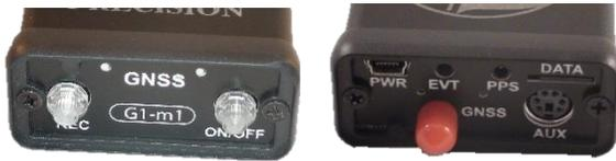
Figure 2: G1-m1™ Receiver CDU and PC Panels
