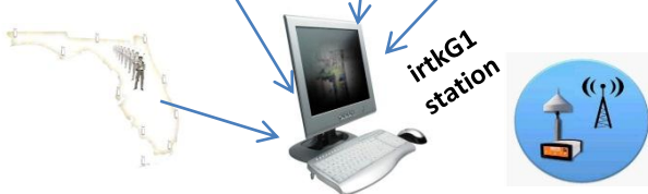
Crew chief in the office communicating with field crews in real time; office is connected to the FPRN and to its own base station through the irtkG1 station
